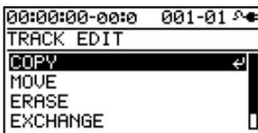
**3** Use the CURSOR [▲][▼] buttons to move the cursor to "EXCHANGE," and press the [ENTER] button.
